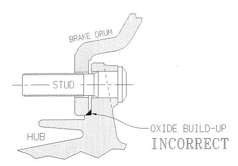
Failure to completely remove the corrosion will prevent the replacement brake drum from contacting the hub flange. When the wheel nuts are tightened, the brake drum can crack. If the crack is not detected the brake drum can fail.
